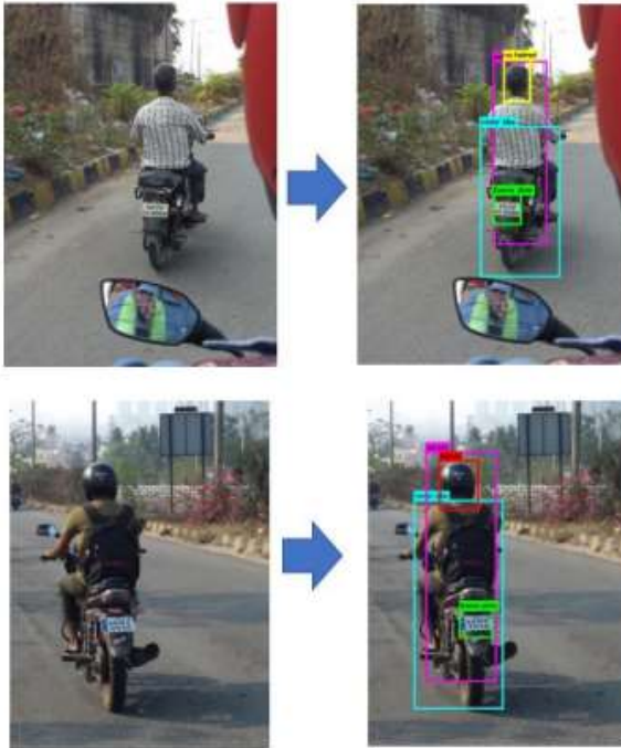
Fig 4: This code removes the license plate from the output of the Object detector. The License plate extraction program is only extracted from motorbikes that have riders who are not wearing a helmet. The code then removes the license plate of motorbikes whose riders wear a helmet.
